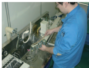
Example of PCB washing
