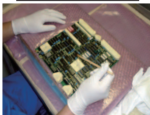
Example of PCB coating
