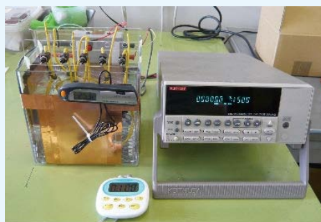
Insulation resistance measurement equipment
