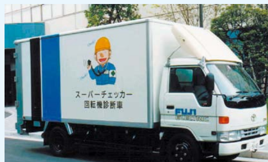
Insulation diagnosis vehicle
