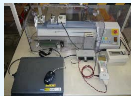
Elongation-at-break test equipment
